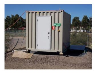
groundwater treatment pack and the primary multi phase vacuum extraction set. Capable of removing separate phase, dissolved phase and vapour phase hydrocarbons from a maximum depth of 5 metres with an applied vacuum of up to -85kPa at a flow rate of up to 1.2 Litres per minute per well.
